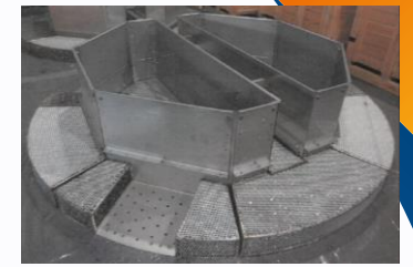
Flashing Feed Gallery, Newly Designed above Bed #1
